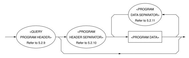
When a <PROGRAM HEADER> of <COMMAND MESSAGE UNIT> or <QUERY MESSAGE UNIT> is followed by <PROGRAM DATA>, a space is inserted between these unit. A <PROGRAM HEADER> indicates the application, function, and operation of the program. If a <PROGRAM HEADER> is not followed by <PROGRAM DATA>, the <PROGRAM HEADER> solely indicates the application, function, and operation to be performed in the device.
