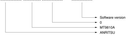
When the manufacturer of the product, whose type name, serial number, and software/hardware version number are Anritsu, 0, and 1 respectively. Sending a common query \*IDN? to a device will return a response message consist of the above four fields.
