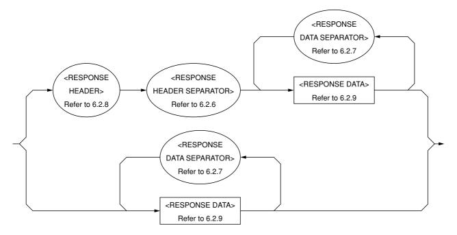
There are two kinds of useage for <RESPONSE MESSAGE UNIT>. One is <RESPONSE MESSAGE UNIT> with header, which returns the result of processing the program-message-set information accurately. The other is <RE-SPONSE MESSAGE UNIT> without header, which returns only the measurement result.
