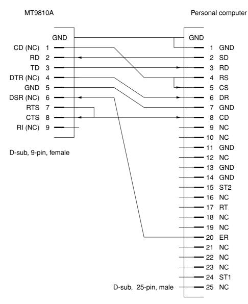
Connection to the external computer with a D-sub 25-pin interface
